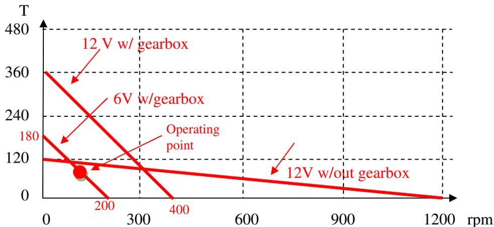
Using the 6V w/gearbox curve,  $T_s=180$  ( $120*3/2$ ) and  $W_{max}=200$  rpm ( $1200/3/2$ ).
